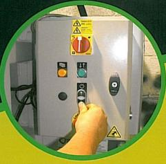
Simple controls with "Bale Full Light" fitted as standard & "Econo Lock" door retention.
